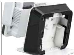
Stable stand due to a die-casting chassis
